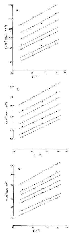
Figure 2 Log-log plot of shear stress vs. shear rate for PC/ABS blends of compositions 100/0 ( $\bigcirc$ ), 90/10 ( $\bigcirc$ ), 70/30 ( $\triangle$ ), 50/50 (×), 30/70 ( $\blacksquare$ ), 10/90 ( $\triangle$ ) and 0/100 ( $\square$ ) at (a)  $210^{\circ}$ C, (b)  $220^{\circ}$ C and (c)  $230^{\circ}$ C
